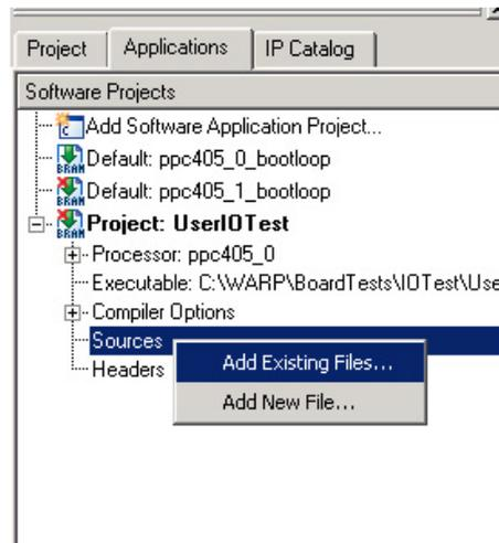
Figure 21: Step 2 – Adding Source Files
