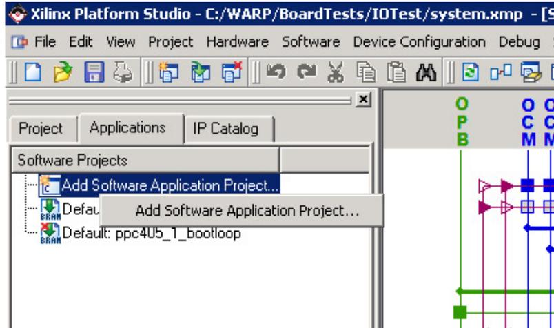
Figure 19: Step 1 – Adding a Software Project
