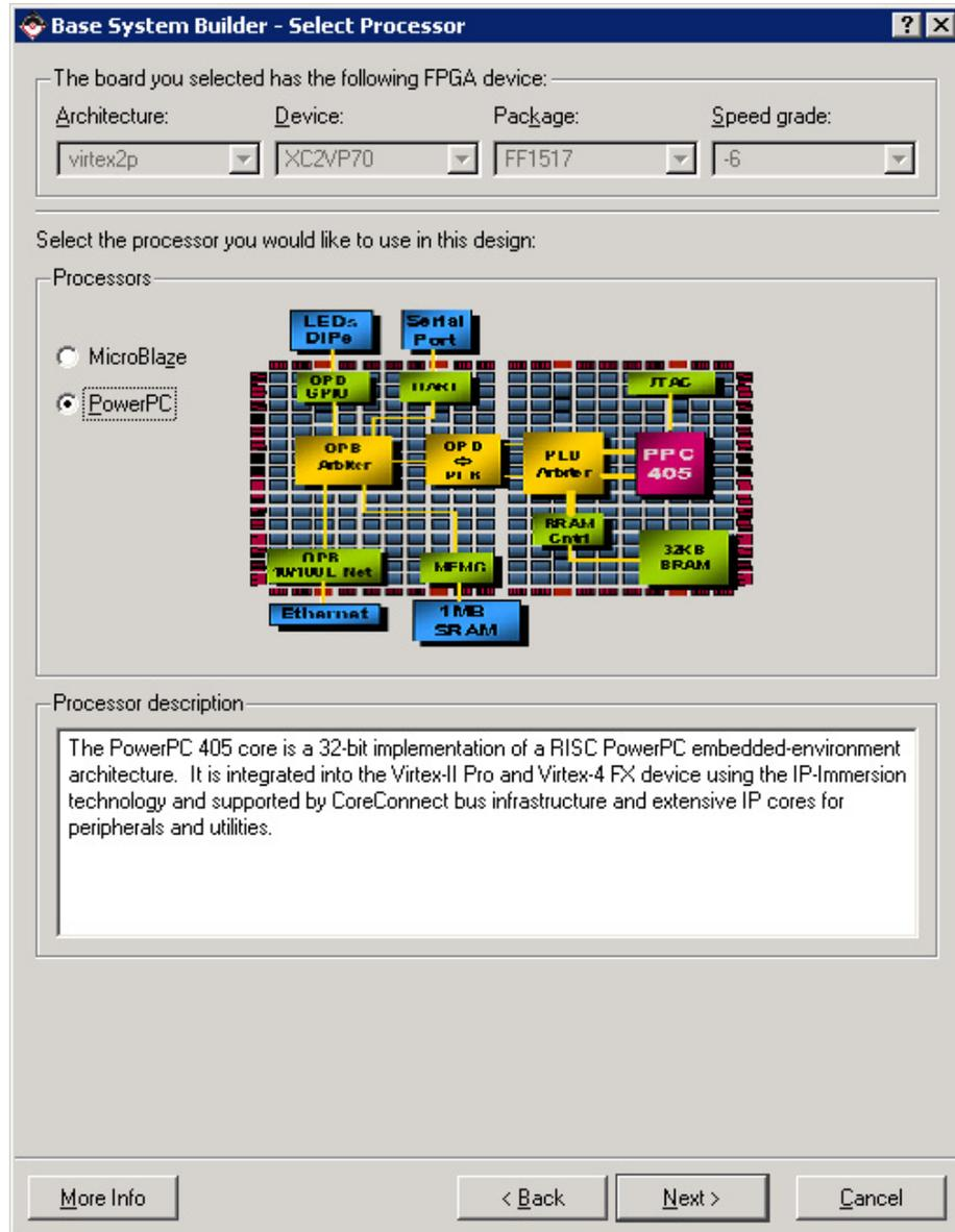
Figure 6: Step 6 – Processor Selection window
