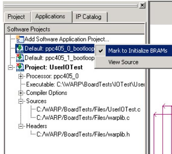
Figure 25: Step 4 – Uninitializing BRAMs for the Default
