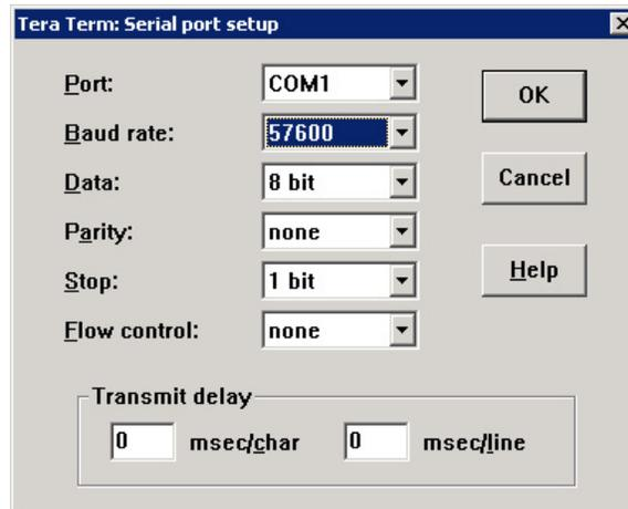
Figure 32: Step 3 – Serial Port Settings
