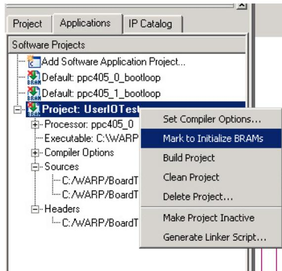
Figure 26: Step 5 – Initializing BRAMs for UserIOtest
