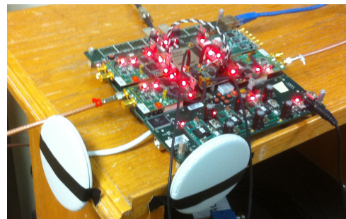
Fig. 2: Full-duplex WARP node with 5 dB directional patch antennas – one pointed towards T_1 and the other towards T_2 .
