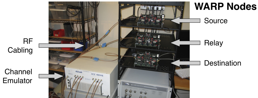
Figure 5.3 : Hardware setup for our experiments, with three WARP nodes and the Azimuth channel emulator.
