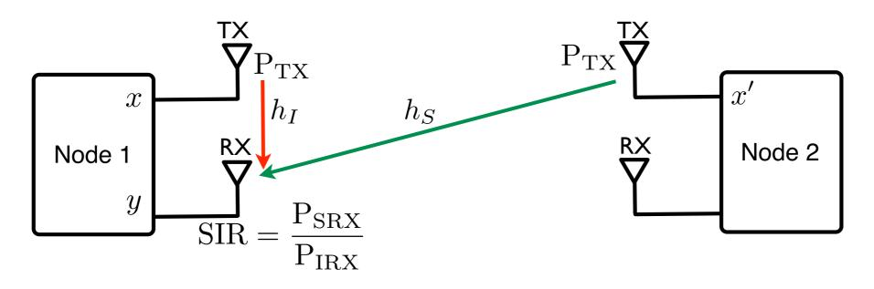
• Achievable sum rate  $ASR = \log (1 + SINR_1) + \log (1 + SINR_2) \qquad SINR_i = \frac{1}{\frac{1}{\alpha_i SIR_i} + \frac{1}{SNR_i}}$
